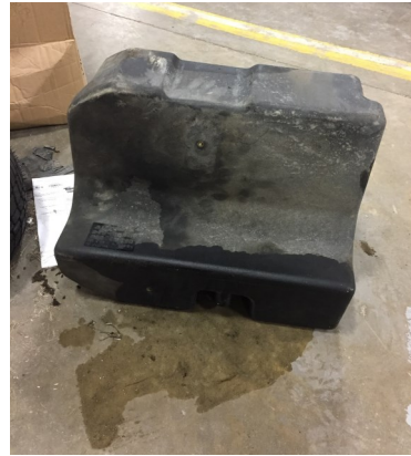
Finally, here is a picture of the old leaking fuel tank.
