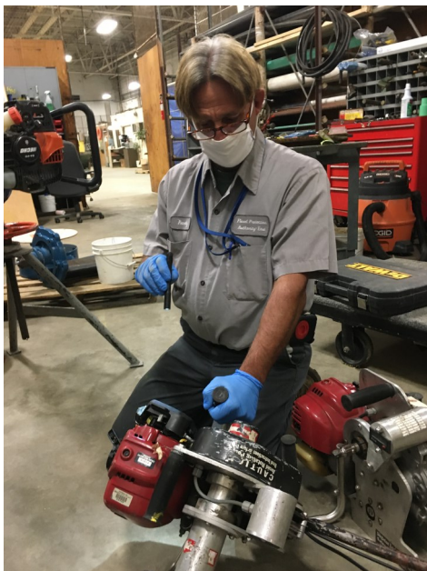
Pictured above: Randy Carter, Plumber/Pipefitter Master, working with a flood valve actuator and ensuring the operability of the flood defense system
