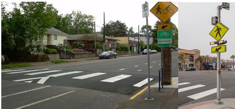
The improvements also include a protected bike lane. Enhanced crosswalks will be installed throughout this stretch of Lakeshore Drive with a raised crosswalk for pedestrians, a pedestrian refuge in the median, and pedestrian traffic signals to alert drivers. The enhanced crosswalks will deter speeding and provide a safer Lakeshore Drive for pedestrians. The project is scheduled to be completed by mid-2021.
